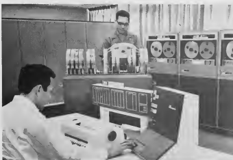
AT THE console of the IBM 1410 Electronic Data Processing System is F. Ruiz, group head in the Accounting Department's Tabulating and Statistical Division. The new Selectric typewriter, right, can print ten characters a second. The special head moves instead of the carriage. Made of plastic, the inexpensive heads can be exchanged for others having a variety of type faces.
